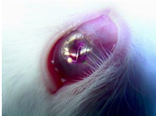
Contact lenses with metal connectors for electronic circuits were safely worn by rabbits in lab tests. (Credit: University of Washington)
